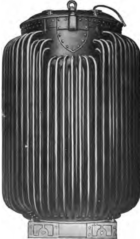
FIG. 79. Additional cooling surface is furnished by the pipes. The oil which carries the heat from the core and coils circulates through the pipes and is cooled. General Electric Co.
